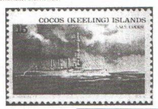
S.M.S. Emden (Cocos Is. SG 24) was built in Danzig in 1908, a cruiser of 3,600 tons, 387 feet long, 44 feet wide, powered by two standing tripleexpansion engines of three cylinders each, a total of twelve boilers giving a top speed of 24 knots; her economic cruising speed was 13 knots. She had ten 4.1 guns - 2 forward, 2 aft, 3 set into each side - and was equipped with torpedoes and mine-laying apparatus.
